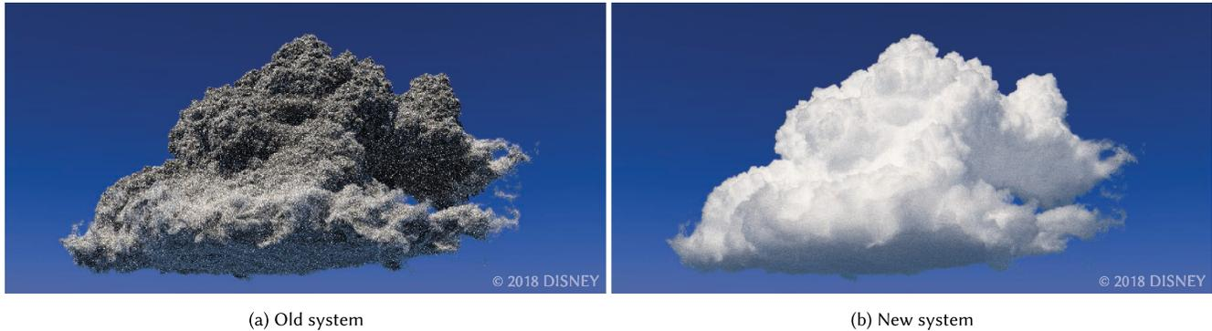
Fig. 12. Equal-time comparison of a cloud rendered using our old *Big Hero 6*-era volume rendering system (left) and our new tracker-based system (right). The old system is limited to 254 bounces (somewhat low-order scattering for high-albedo volumes), yet still produces a noticeably noisier image than the new system. The new system produces a less noisy image while also supporting efficient high-order multiple scattering.
